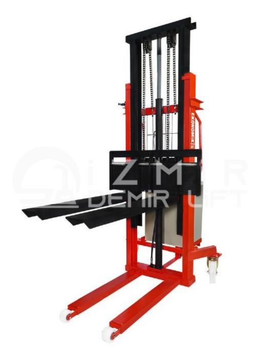
Driving Type : Manuel Lifting Type : Electric Operating Voltage : 220 Voltage- 380 Voltage Capacity: 1500 kg Machine Lift Height : 2500 mm Closed Height of the Machine : 1800 mm Open Height of the Machine : 2800 mm Machine Width : 115 cm Fork Lenght: 115 cm Fork Width :140 mm Forks Far Right / Far Left ( Overall Dimension): 90 cm Machine Weight : 340 kg Wheels : Polyamide Brake : Manuel The Reels Are Made of Cast Material. Forks Can Be Manufactured As Fixed or Mobile
